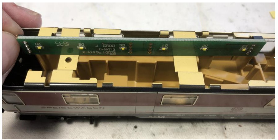
Fig. 9 Checking LED clearance with braces.
